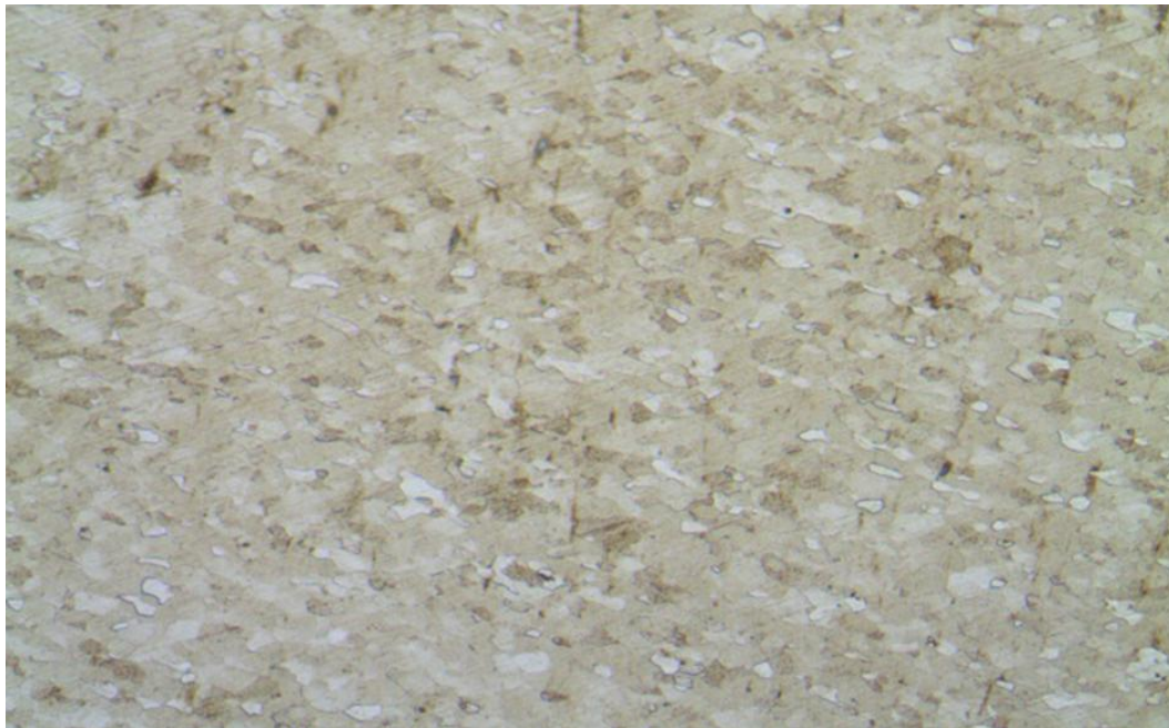
Figure 5. Optical microscopy picture of typical AISI D3 tool steel
