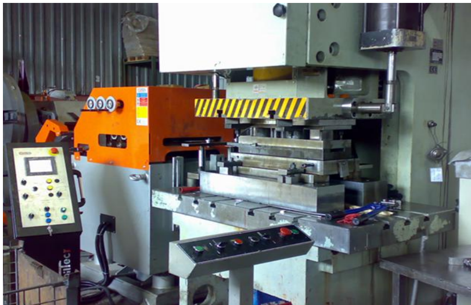
Figure 3. Experimental equipment of blanking sheet metal process
