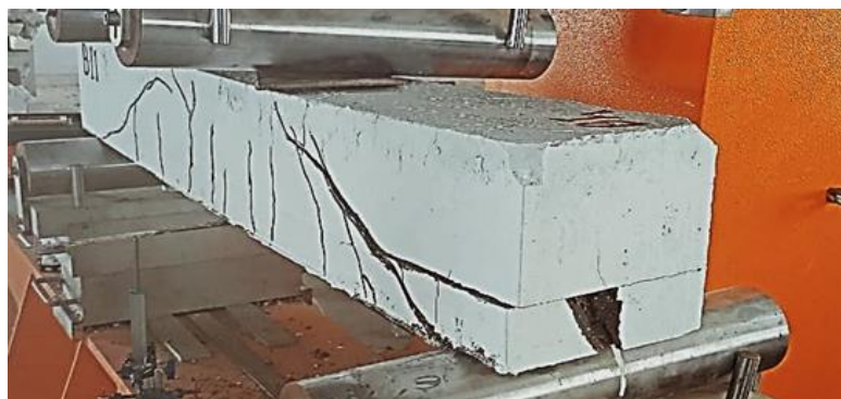
Figure 10. Slip concrete layer in BI1 beam
