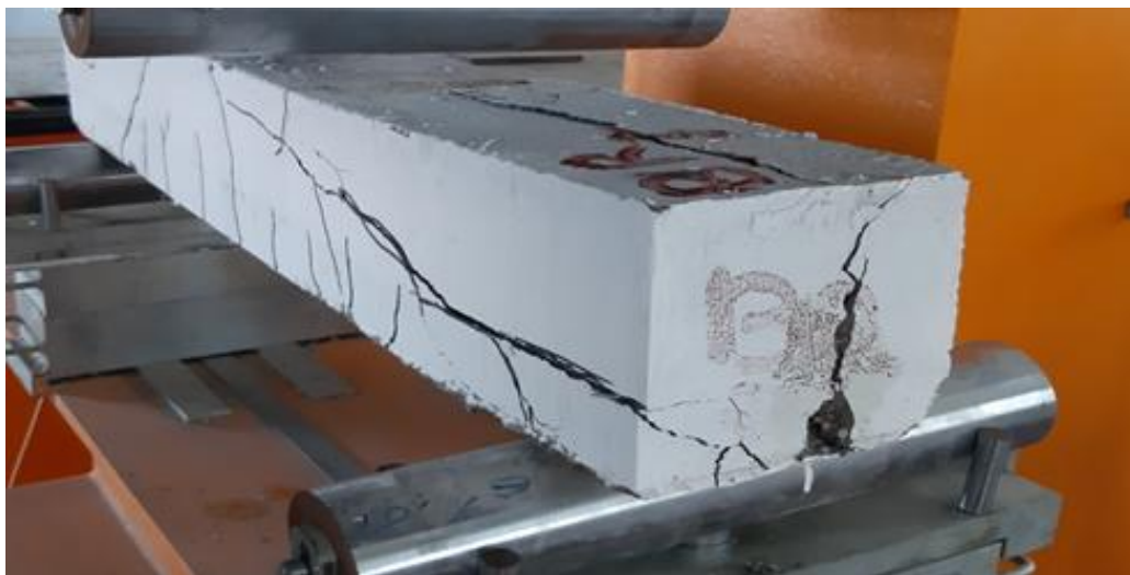
Figure 8. Slip concrete lower layer in BR3 beam
