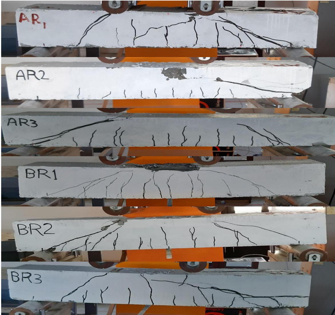
Figure 7. Crack pattern of beams with rectangle shear connector
