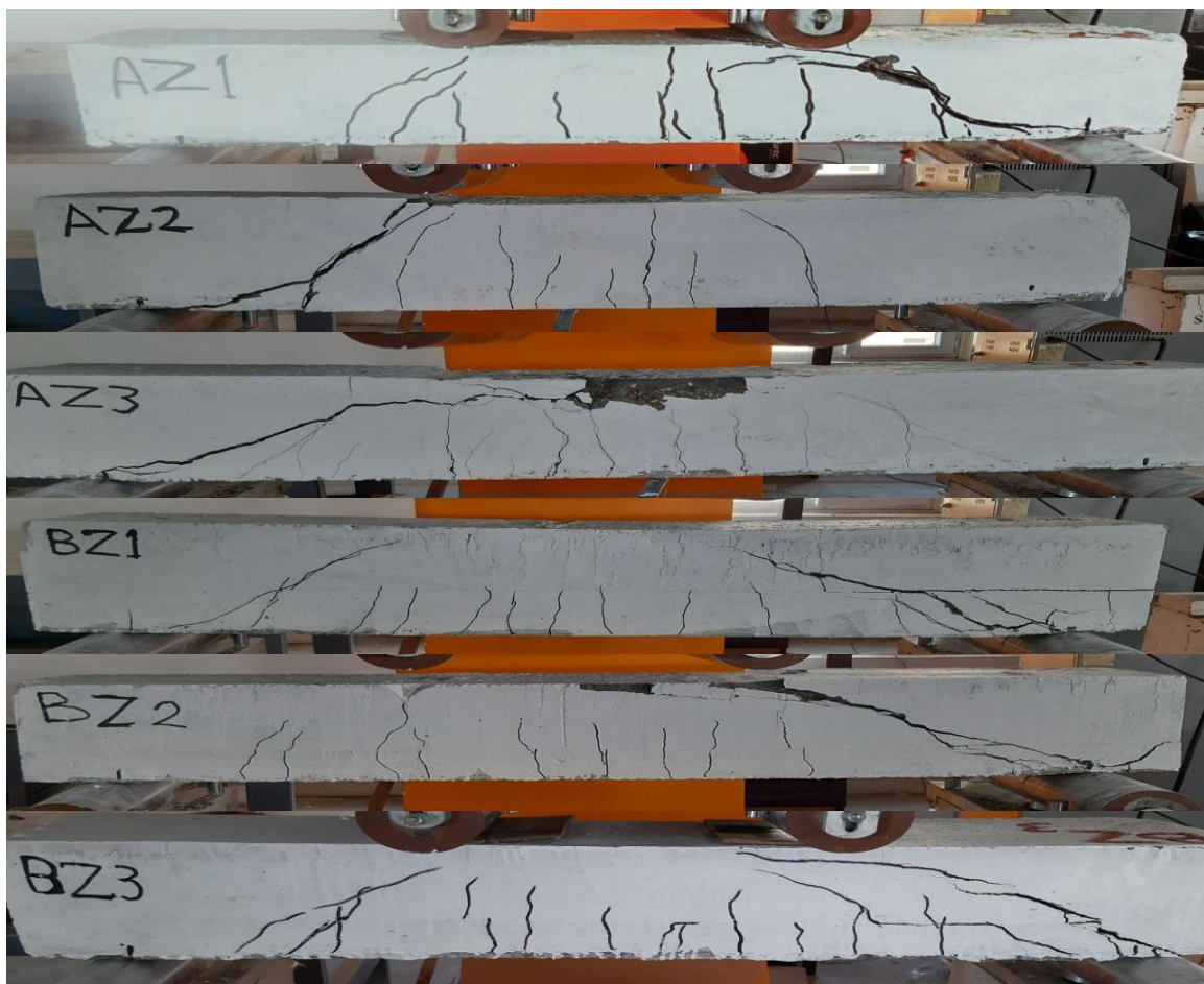
Figure 13. Crack pattern of beams with Z- shear connector
