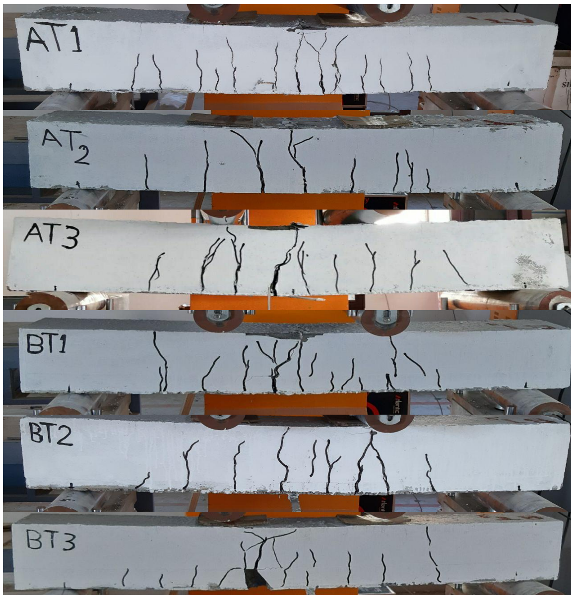
Figure 14. Crack pattern of beams with truss- shear connector
