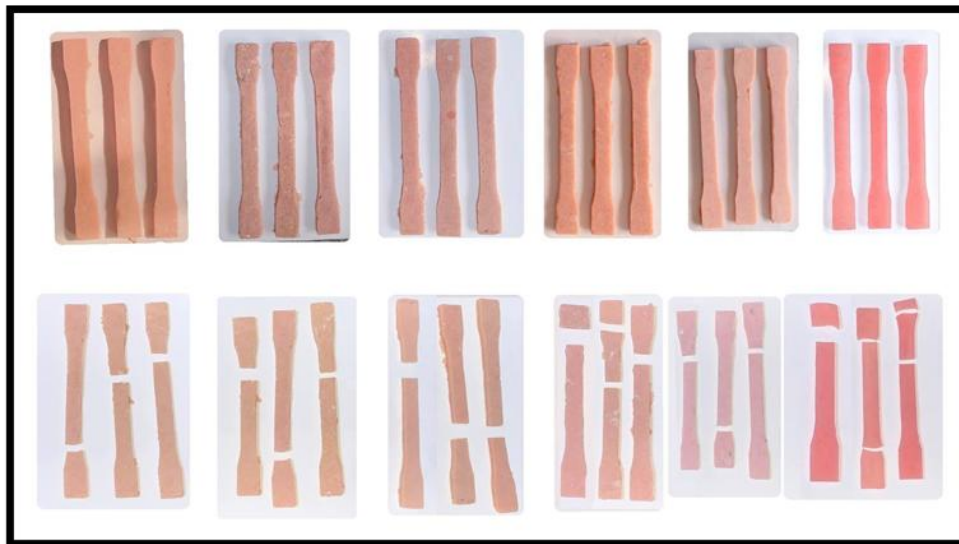
Figure 4. Shape the sample before and after the tensile test
