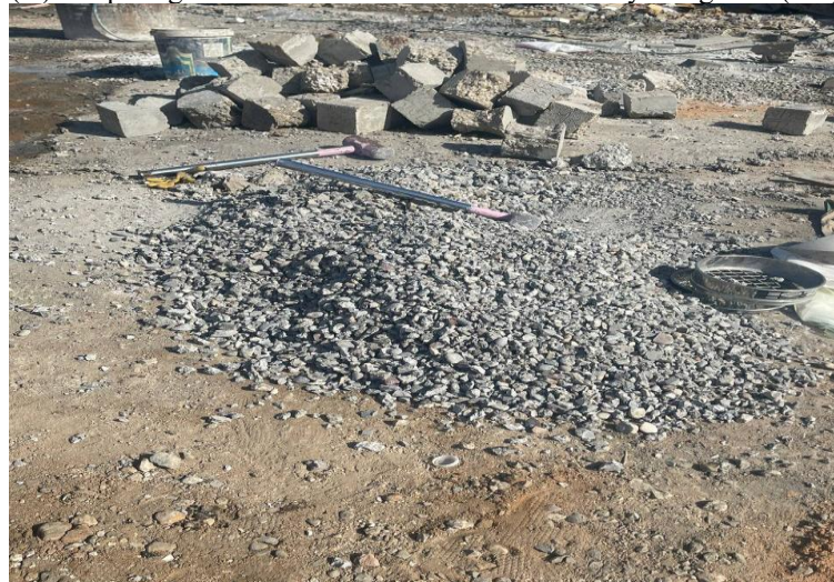
(B): Manual method (hammer) used to obtain recycled gravel
