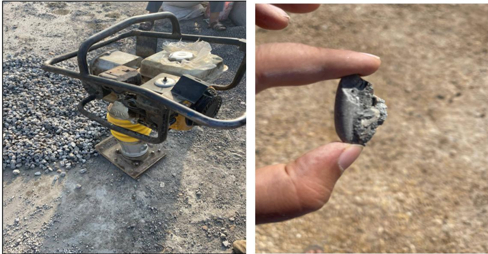
(C): Mechanical method used for obtaining recycled aggregates with sieve grades similar to conventional normal aggregates using mechanical device
