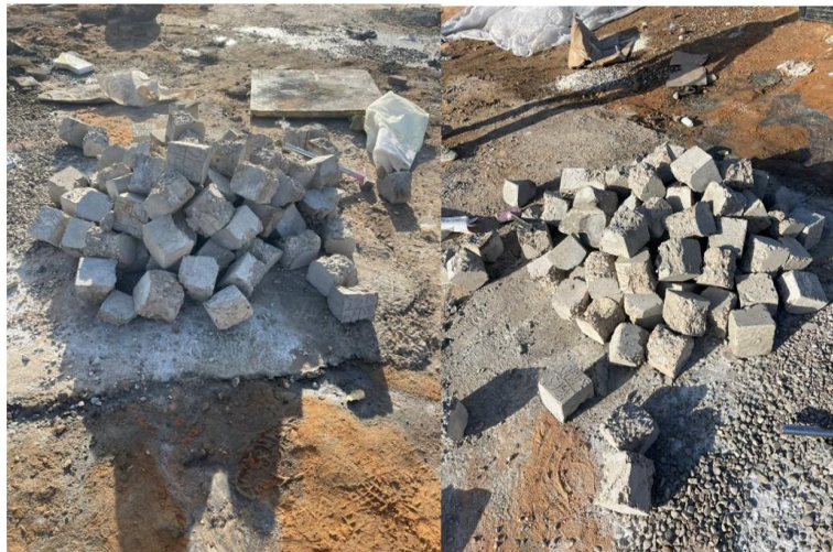
(A): Preparing old concrete cubes used to obtain recycled gravel (RA)
