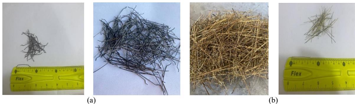
Figure 1. Steel fiber (a) manufactured steel fiber, (b) recycled steel fiber from a tire.
