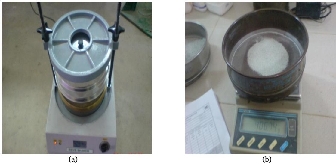
Figure 2. Equipment for Sieve Analysis Test; a) Sieve set with shaker b) Weighing machine and pan
