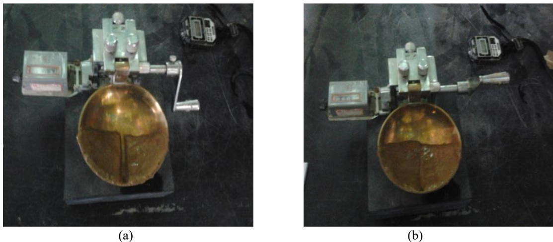
Figure 2. Casagrande cup for Liquid Limit test. (a) The sample was divided into two halves using a grooving tool in the Casagrande cup. (b) The two halves of the soil were in contact after being dropped by turning the handle of the apparatus.
