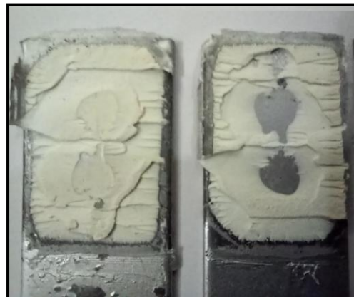
Figure 20. The non-perforated single-lap joint specimen's mode of failure
