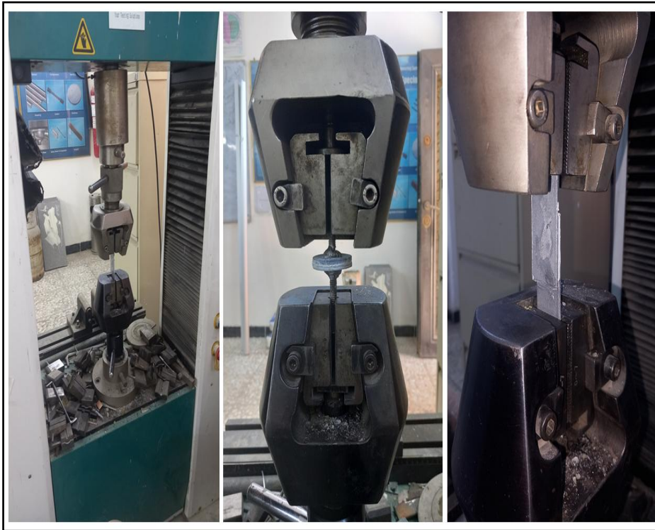
Figure 11. Universal testing machine
