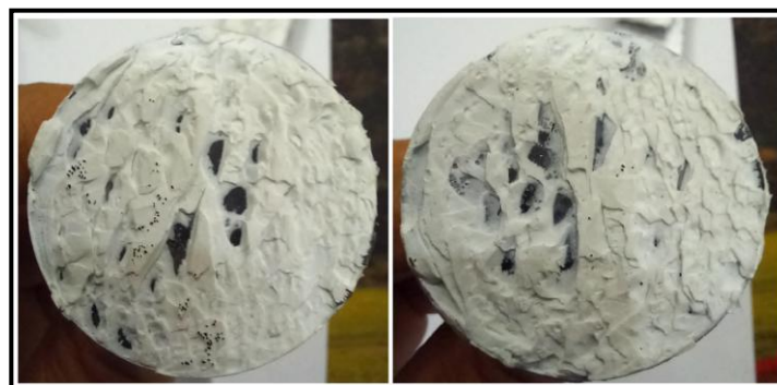
Figure 15. The failure mode of a non-perforated butt-joint specimen
