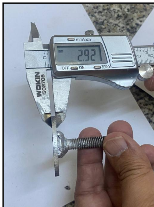
Figure 8. Regulate the specimens' thickness.
