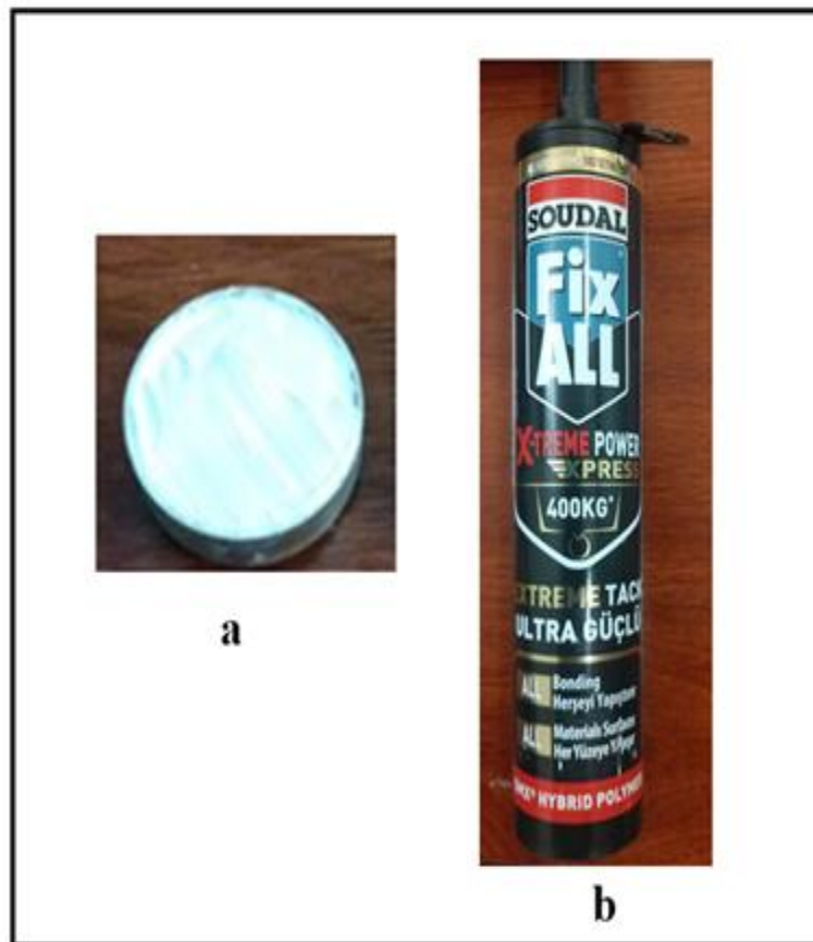
Figure 1. (a) Appearance of MS hybrid polymers, (b) Trade name and packaging of the adhesive
