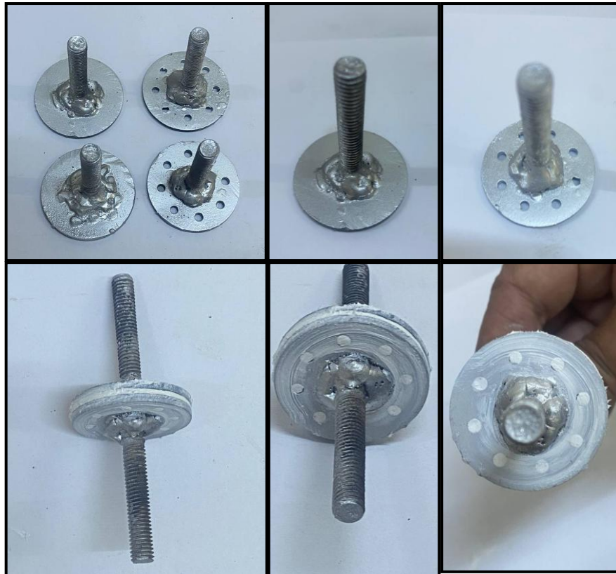
Figure 9. The specimens of butt-off
