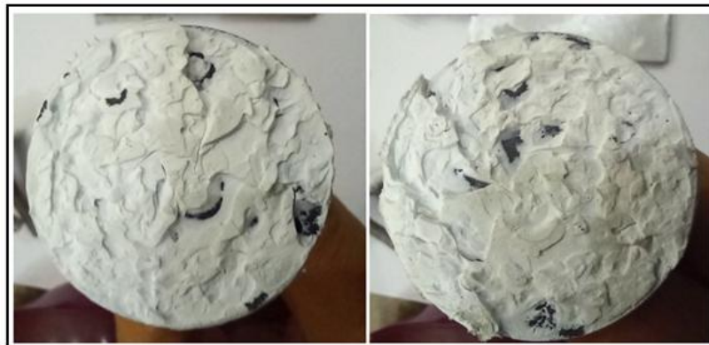
Figure 14. The failure mode of a perforated butt-joint specimen
