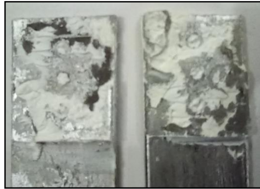
Figure 19. Failure of the single-lap perforated joint specimen
