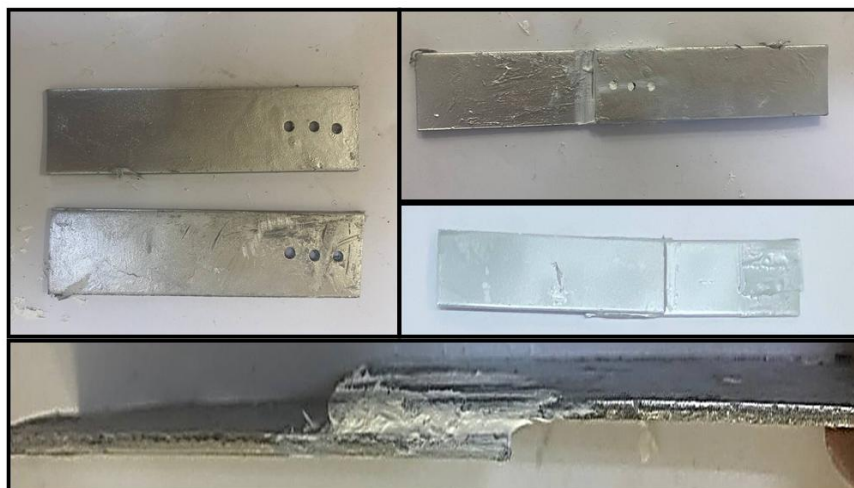
Figure 10. The specimens of a single lap joint
