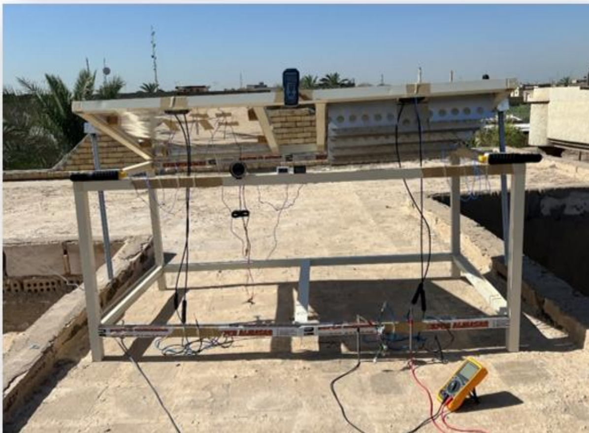
Figure 3. Experimental work on cooled PV panel and reference panel
