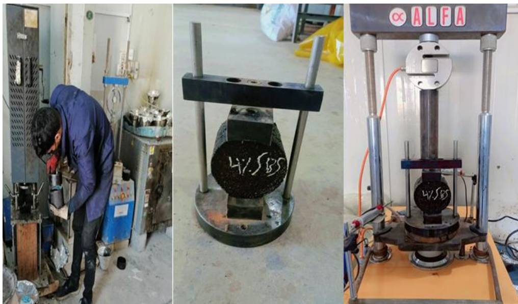
Figure 10. Laboratory tests of ITS devices and specimens.
