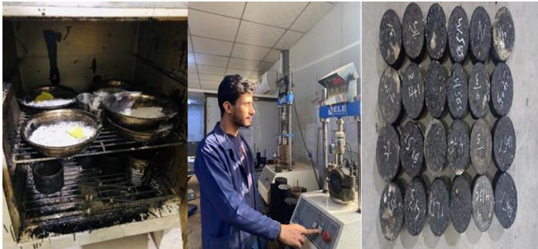
Figure 8. Laboratory tests of Marshall in the highway lab at the University of - Al- Qadisiyah
