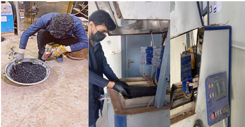
Figure 11. Conducting the (WTT) to evaluate the performance of modified asphalt mixtures
