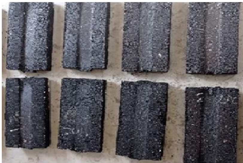
Figure 19. Effect of rut depth under wheel tracking test on asphalt samples
