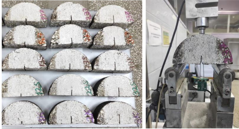
Figure 2. Semi-circular bending (SCB) test specimens and experimental setup
