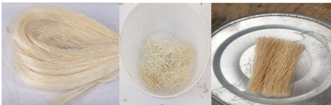
Figure 1. a) Sisal fiber, b) length sisal fiber 3cm, c) length sisal fiber 7cm.
