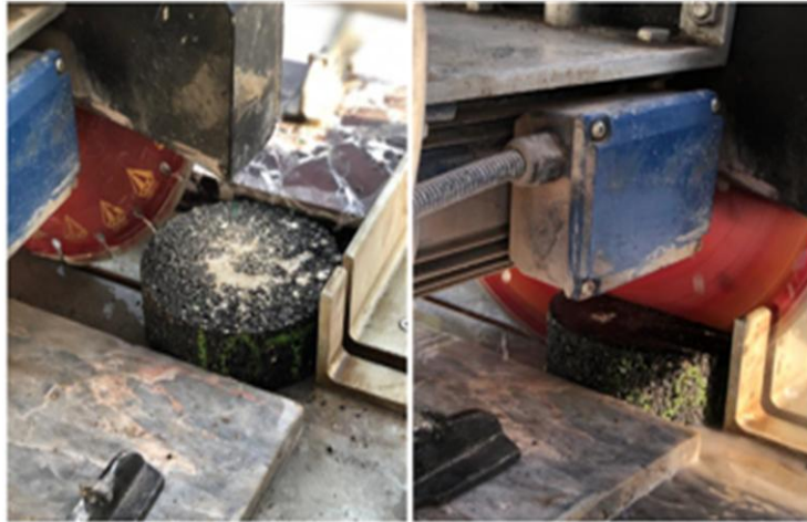
Figure 4. The preparation of a typical SCB sample
