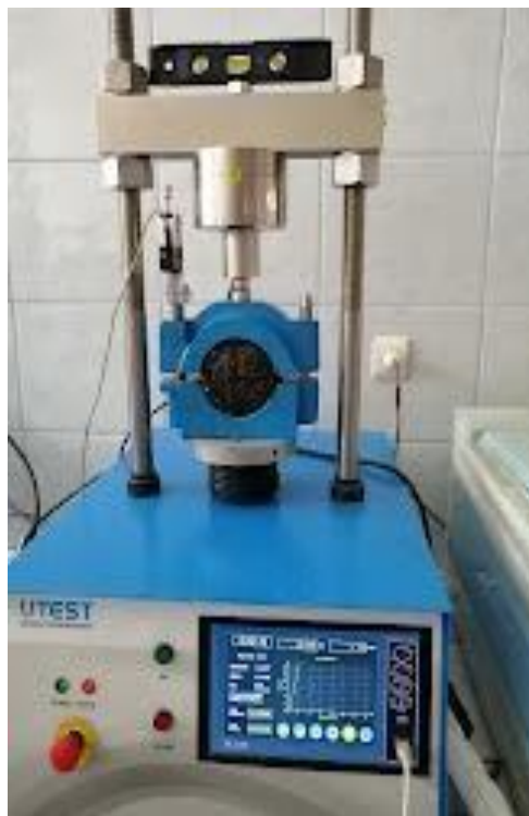
Figure 4. Performing Marshall stability and flow test
