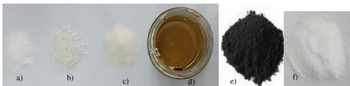
Figure 1. Additives used in the study: (a) SBS polymer, (b) Elvaloy, (c) 611 polymer, (d) PPA, (e) CR, (f) 701 polymer
