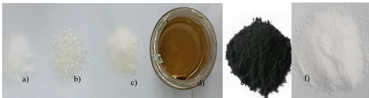
Figure 1. Additives used in the study: (a) SBS polymer, (b) Elvaloy, (c) 611 polymer, (d) PPA, (e) CR, (f) 701 polymer
