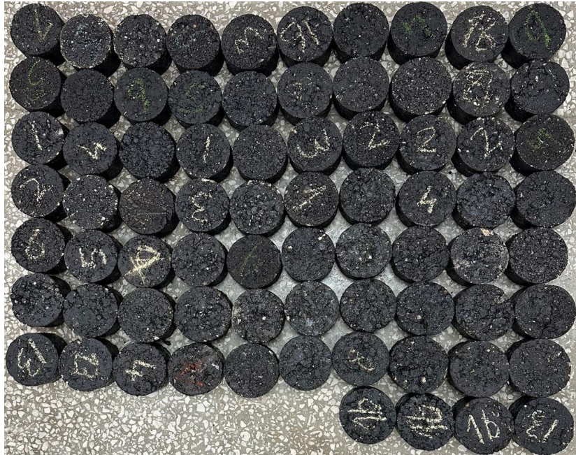
Figure 2. Asphalt mixture samples prepared during the project study
