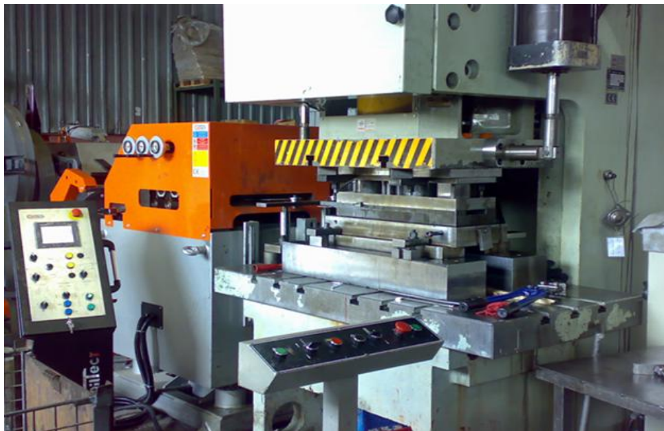
Figure 3. Experimental equipment of blanking sheet metal process
