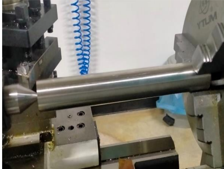
Figure 1. A standard lathe machine used for machining stainless steel through carbide insert
